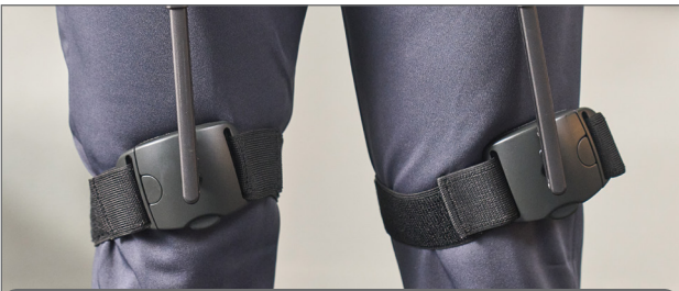
Excessively extended frame, loose leg strap, and tilted buckle
